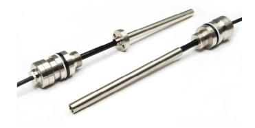
**SPECIFICATION** Dimensions Body Diameter: Body Length: Probe Length: Ø27 mm 41.5 mm calibrated travel + 28 mm (nom.) Target Tube Length calibrated travel + 30 mm For full mechanical details see drawings P116-11 **Independent Linearity**  $\leq \pm 0.25\%$  FSO @ 20°C - up to 600 mm < = 0.01%/°C Gain &
